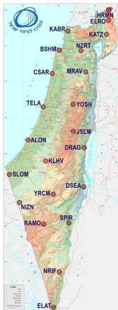
Figure 1: The primary horizontal control in Israel is a network of 21 CORS
