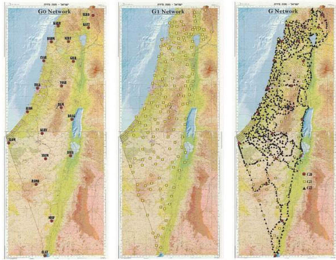
Figure 2: The first three levels of the Israeli geodetic infrastructure
